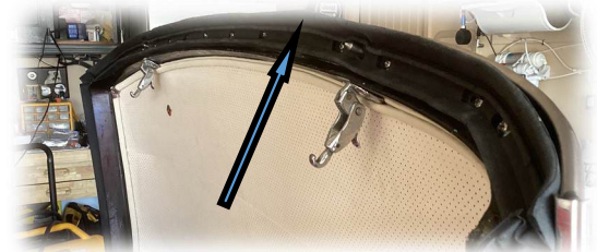
Final Trim and Rubber Gasket with new internal mount bars assembly completed
