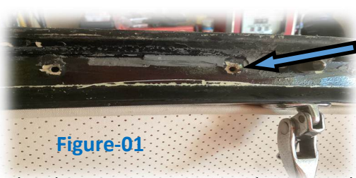
Fiberglass to gasket mount area, underneath is the metal mounting bar
